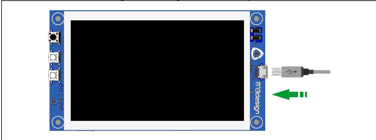
Figure 9. Connecting the board to the computer
