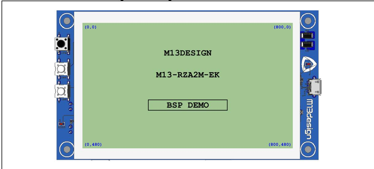
When the board is rotated 180° (still in landscape view), the screen will rotate its display information to match the user’s view. In order to this, the application checks the changes in the accelerometer’s Y axis and rotates the display if a threshold is reached. In addition, you will also have access to the rotation value through the console as shown below in [Figure 18](#). Note that the board will recognize two rotation position, **ROTATION\_ZERO** or **ROTATION\_180**.
